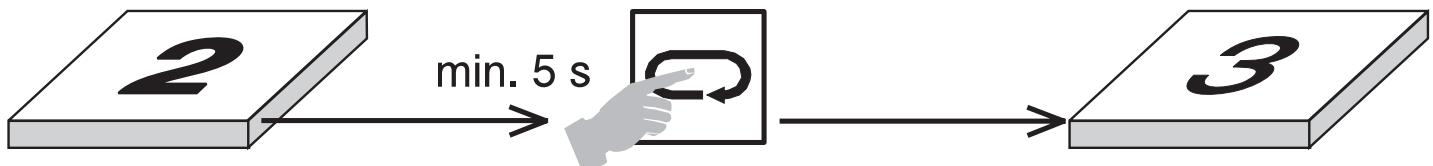
After transition to configuration level, **Con** in the 1st and configuration word **0x00** in the 2nd display line are indicated.
