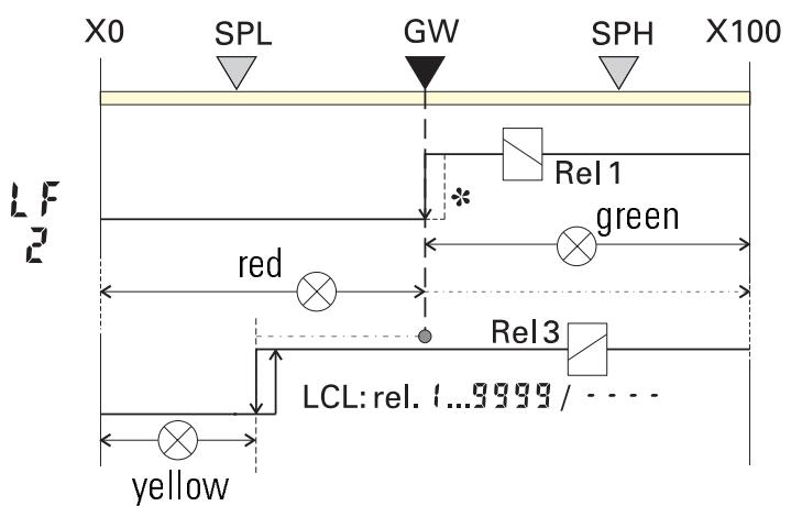
When leaving the alarm or limiter range, relay 1 is locked. Reset (\*) can be done as described (→ **Reset**), however, the external contact is evaluated statically. A continuously closed contact will cause immediate reset.
