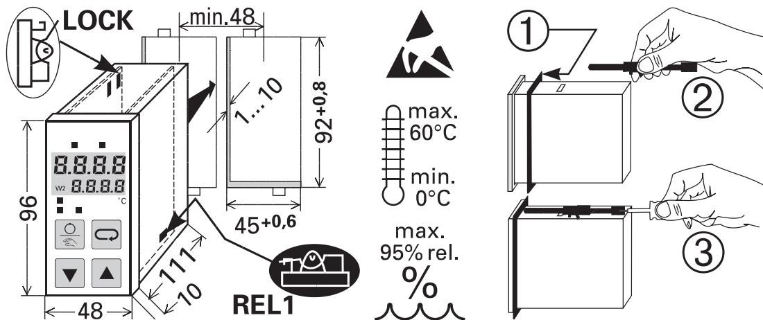
With a sealing ① between controller front and panel, the panel reaches protection mode IP 54. For access to the S.I.L. switches REL1 and LOCK, remove the controller module from the housing by pulling it forwards at the top and bottom cut-outs.
