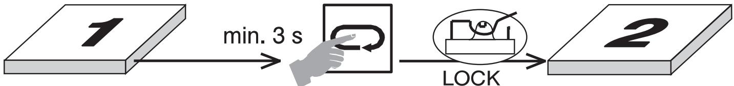
**With S.I.L. switch **LOCK** open, transition to parameter level is permitted.
