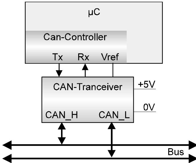
With CAN bus, the nominal CAN bus levels are described as Recessive (nominal voltage 2,5V for CAN-H and CAN-L) and Dominant (nominal 3,5V for CAN-H and 1,5V for CAN-L).
