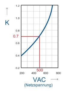
\*I2T are multiplied for K value in function of Vac at 500V K is equal to 0,7 (ex:12400 X 0,7 = 8680). At 660Vac K is equal to 1.
