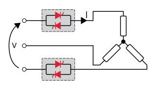
Delta wiring with resistive load (control on two phases with PMA-Relay C-2PH)
