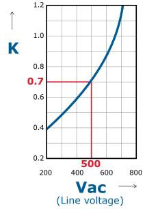
\*I2T are multiplied for K value in function of Vac at 500V K is equal to 0,7 (ex:105000 X 0,7 = 73500). At 660Vsc K is equal to 1.
