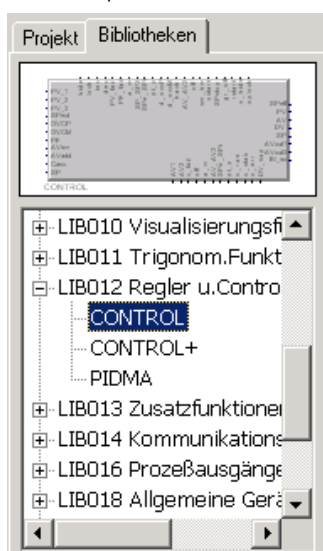
Fig. 49: Programmer project: Selecting controller "CONTROL"
